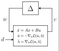
some unmeasurable and unpredictable disturbance, predictive methods like MPC might become impractical. A promising remedy is to design optimum seeking reactive controller, leading to the concept of feedback optimization. Here, the idea is to choose a suitable gradient flow that incorporates feedback measurements, such that the optimization algorithm becomes the controller itself. Case studies show promising results, e.g. for the application on power grid systems.
